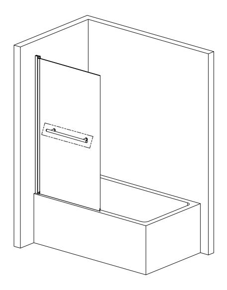
EXTERNALLY SILICONE SEAL THE WALL PROFILE WHERE IT MEETS THE WALL AND ALONG THE BOTTOM OF THE BLACK PROFILE. ALL IN A CONTINUOUS BEAD. DO NOT SILICONE INSIDE THE BATH SCREEN
